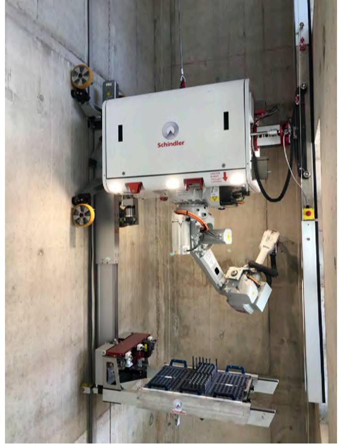
Kurulum robotu Schindler R.I.S.E. alıřırken; Schindler'in izni ile Installation robot Schindler R.I.S.E. at work; courtesy of Schindler
